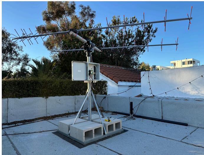
The best antenna for use on a tracking mount will usually be a circularly-polarized Yagi-Uda (aka “Yagi”). Most good choices will be around 7+ft long, offering peak gain of 12dBi or more. They will generally be mounted around the middle of the beam.
